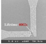
Prediction and experimental results of wiring life and wiring location (left: prediction, right: experimental results)
